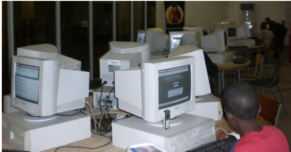
Innovative round tabletops designed by SchoolNet Namibia reduce computer failure rates, as cables are fed through the centre of the table.
